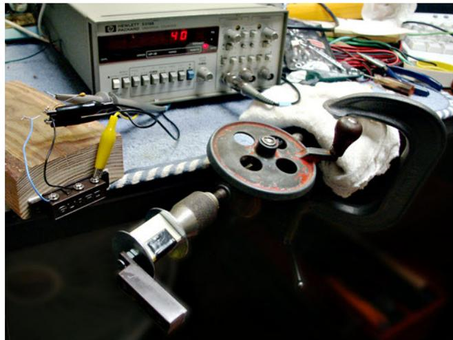
The thing was, I might never need this machine again, depending on how this went. After thinking about it, I decided to try rigging-up a simple winder, using my Dad's old 1/4" hand drill, as **shown above right**. I used a standard lab counter, operating in totalize mode, to count the turns.
