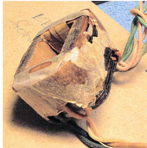
secondary. **At right**, we zoom-in on the center two leads (primary and HV CT). Notice that there are two HV wires because that is the center of the two halves of the HV secondary. The HV secondary wire looks thin compared to the already-thin primary wire. Varnish pervades the transformer.
