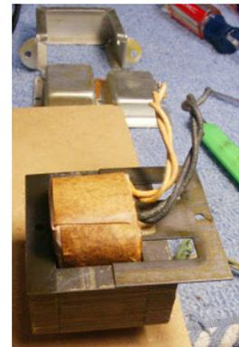
new tip seem to work well. You can see the knife I used, **at right**. The first lamination will be the most difficult. You will notice that there are two types of laminations (**hereafter “lams”**). The E-shaped pieces butt against I-shaped pieces. The technique is to work the blade under the corner of an E-lam. They are cemented together by a varnish.
