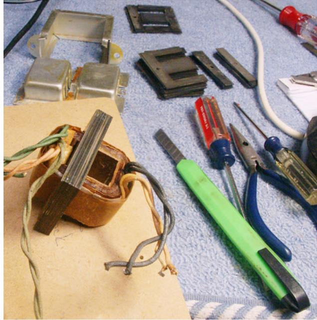
Try not to bend them so much that they are no longer flat, though. There is a tradeoff between speed and how much you end up bending them. In the end, we will want them to be as compact a bundle as possible, to optimize the quality of the transformer. It took me about an hour to disassemble the ST-84 transformer—removing about 36-lams.
