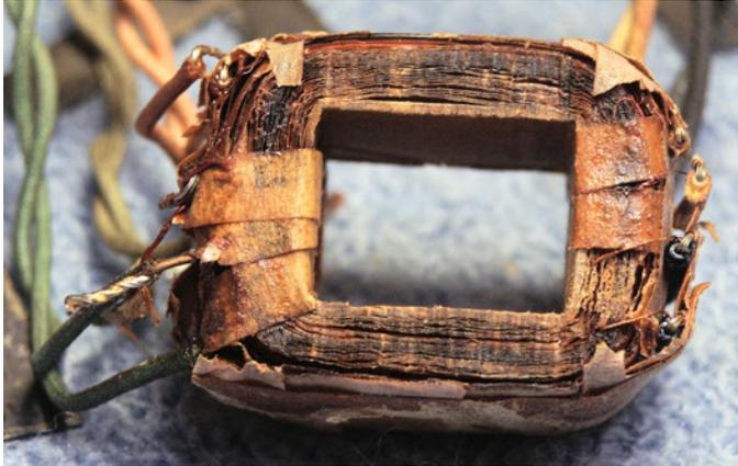
In the view **at left**, you can see the green filament leads going to thick winding wires. The light green leads are another 6.3V filament winding going to somewhat thinner winding wire. The HV leads at the upper left were once red but have faded to yellowish orange. If you look carefully at
