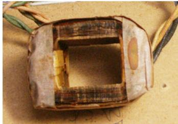
When you are finished with the lams, you will have the bare transformer coil, as seen **at left**. Let's digress for a moment to take a look at that. You can see the blackened edges of the windings, indicating that my unit had burned. The windings are separated by and covered by layers of paper, impregnated with varnish.
