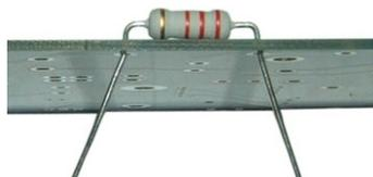
After inserting the component leads into the respective holes on the board, bend the leads outward slightly. This will prevent the component from falling out of the board when it is turned over for the soldering procedure.
