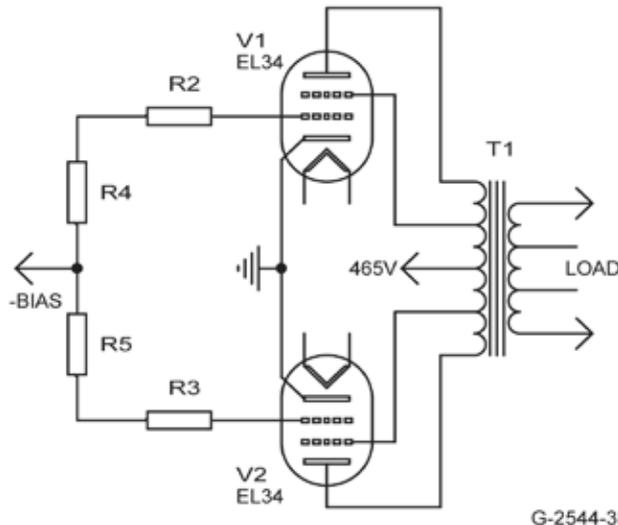
**FIGURE 4: Screen stability resistors.** In spite of operating the screens at their design maximum voltage rating, at the same voltage as the plate, in a fixed bias design, and from a very low impedance power supply (Fig. 1C with a regulator), these high transconductance tubes will now maintain screen stability under all signal conditions.
