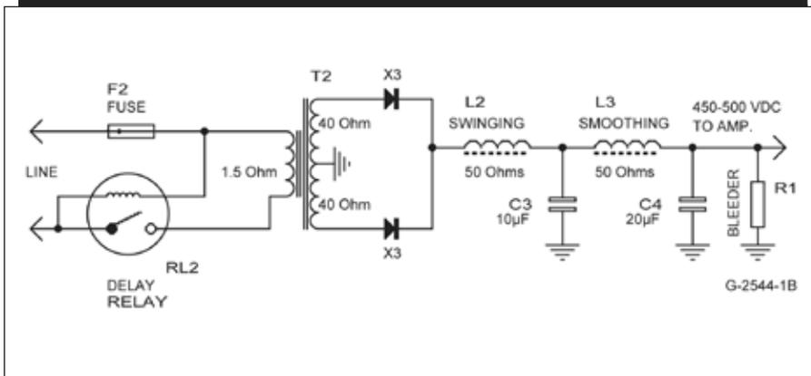
**FIGURE 1C: Modern supply design. The internal resistance of this supply is only  $\approx 28\Omega$  with significant peak current reserve.**
