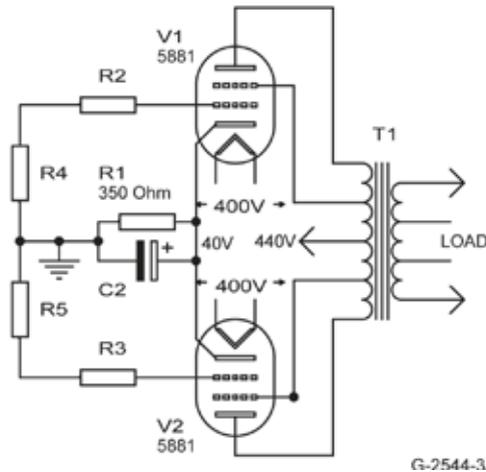
**FIGURE 3B: Fixed bias ultralinear output stage. Same conditions as in Fig. 3A except for the use of fixed bias and higher transconductance tubes. This design has only conditional screen stability, remaining acceptably stable only when operated from a power supply with characteristics as shown in Figs. 1A or 1B. Operating this design from the supply in Fig. 1C will promote output tube arcing.**
