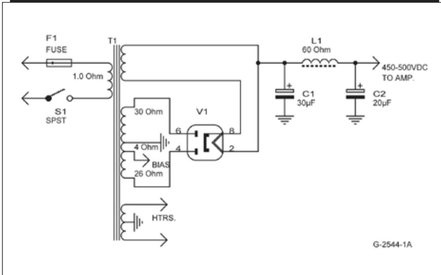
**FIGURE 1B: Classic supply with better regulation. The internal resistance is now  $\approx 140\Omega$ , but the combined bleeder and choke action effectively reduces this to  $\approx 85\Omega$ .**
